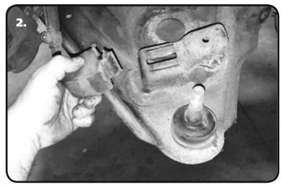
**2.** Remove the OEM Bumpstop from the lower control arm. Put a small pry bar under one end and pry it up, work your way to the other end prying it out as you go.
