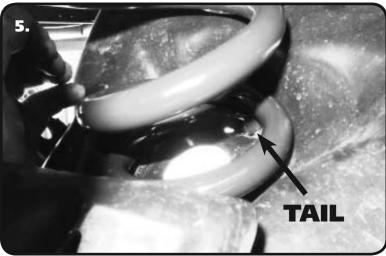
**5.** Insert the CoilSpring/Seat combo into the OEM coilspring pocket aligning the Rivet in the notch of the Upper Seat. Twist the spring on the Upper Seat to get the bottom of the CoilSpring lined up with the receiver in the control arm. The end of the CoilSpring needs to be nested into the receiver area of the Control Arm.
