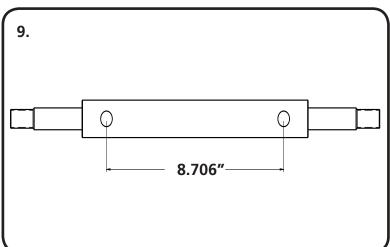
**9.** The Lower Cross Shaft has 2 different locating Hole patterns. These StrongArms use the 8.706"" center to center locating holes. The Pin in the Cross Shaft Saddle that was pointed out in **Image 8**, will locate into these Holes. Use the OEM Hardware to attach the Lower making sure the Locating Pin is in the 8.706" center to center Holes.
