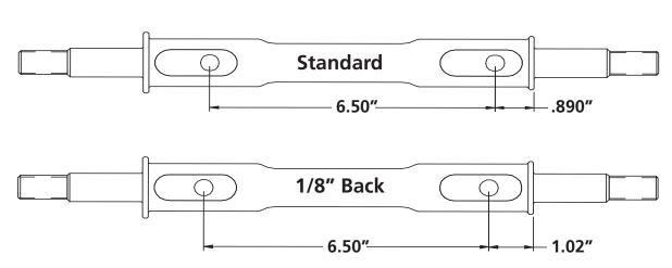
These StrongArms come equipped with a changeable caster slug setup. This allows you to add or remove caster from the front suspension, if desired. The caster slugs that come supplied in the kit are setup to provide approximately 5 degrees of caster. The caster slugs allow you to add or remove caster without having to use a stack of shims. If more or less caster is desired, optional slugs can be purchased from Ridetech or your Ridetech dealer.
