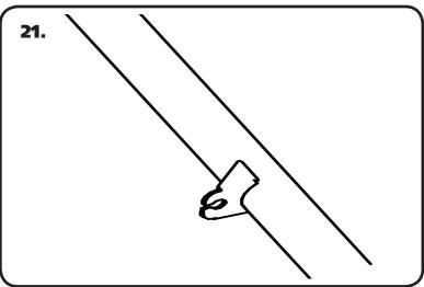
**21.** The StrongArms have a tab for the emergency brake cable. Install the cable into the tabs and hook the cables back up.
