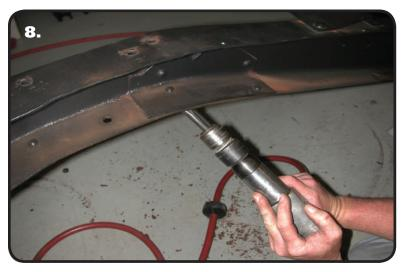
**8.** The lower rear rivet on this reinforcement plate must also be removed to mount the notch.
