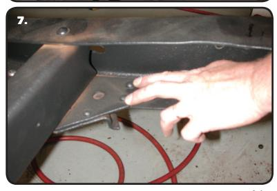
**7.** On the driver side of the rear frame cross member; these two rivets must be removed before installing the "C" notch. Also, remove the factory panhard mount.
