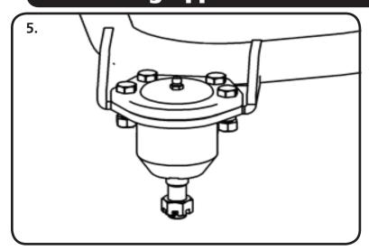
**5.** Install the balljoints into the upper control arm with the hardware supplied with the balljoint. The upper balljoint goes in from the top side of the control arm. The gussets on the balljoint plate point up. Torque the mounting hardware to 29 ftlbs.
