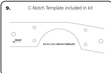
**9.** Use the supplied "C" Notch template to mark out the frame for cutting. Before cutting out the frame, support the frame in front of and behind the "C" Notch area. We suggest doing one side at a time. The "C"Notch template has an arrow pointing to the front of the truck. Use the 5/8" holes to locate the template of the frame.
