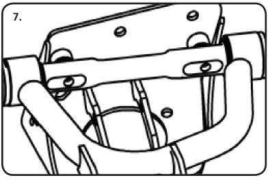
7. Install the caster slugs into the cross shaft. The long side of the caster slug goes to the front of the truck. The cross shaft is attached to the truck using a 7/16" USS Flat Washer & 7/16" Nylok Nut. The drivers side is shown in figure 8. Slide an Aluminum T-washer on each end of the shaft up against the bushing with the FLAT side Toward the locknut. Now install a 5/18"-18 locknut on the shaft. This nut gets snugged up. You want the suspension to be able to move freely.
