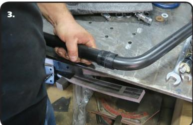
**3.** The Delrin Liner is split on one side to ease installation. We found it easier to install by opening up the Liner enough to slide it onto the end of the SwayBar, then sliding it into position. It will open up and slide over the curves in the Bar. Install a Liner on each side of the SwayBar in the approximate location they will need to be when installing the SwayBar on the Truck.
