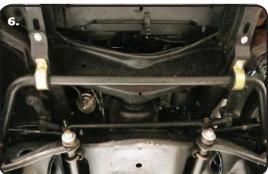
**6.** Hold the SwayBar into position on the truck with the SwayBar arms below the tie rods. Align the holes in the Bushing Straps with the holes in the Frame Brackets. Install a 3/8" Flat Washer on (4) 3/8"-16 x 1 1/4" Hex Bolts and insert them into the holes. Install a 3/8" Flat Washer and 3/8"-16 Nylok Nut on each Bolt. Center the bar in the bushings before snugging up the hardware. Do **NOT** completely tighten the Hardware. It will be left partially loose until the End Links are installed.
