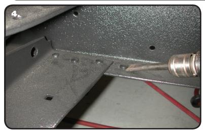
**4.** The factory trailing arm frame cross member will be replaced with the tubular one supplied. To remove the factory cross member, the rivets must be removed. The easiest method is to chisel them off with an air hammer. Then use a hammer and punch to drive the rivets out.
