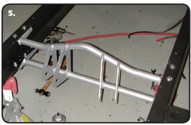
**5.** Install the new cross member with the trailing arm flanges towards the rear. The cross member is bolted to the bottom side of the frame rails using 10 - 7/16" x 1" bolts, 10 - 7/16" Nylok nuts and 20 - 7/16" flat washers. It may be necessary to enlarge some of the holes with a 7/16" bit.
