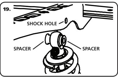
**19.** Install a spacer on each side of the upper Shockwave/Coilover. Slide the assembly into the upper bridge from the bottom side. If your shock has an adjuster knob position it so that the knob points toward the center of the truck. Line up the hole in the spacers with the hole in the upper shock bridge and insert 1/2" x 3 1/4" bolt and install 1/2" Nylok nut.
