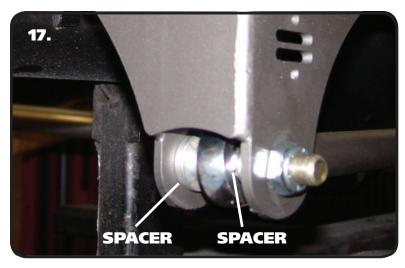
**17.** Install the Panhard bar into the frame bracket using a 70013334 Spacer in each side of the R-Joint end. The Panhard bar is attached using 5/8" x 2 3/4" bolt and a jam Nylok nut.
