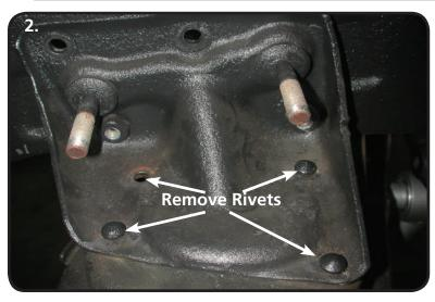
2. The factory upper control arm mount will need to be removed from the frame. There are 4 bolts attaching it to the frame rail with 4 rivets attaching it to the crossmember. There are several methods that can be used to remove the rivets from the crossmember. One way is to cut a "+" in the head of the rivet and chisel the 4 pieces of the head off the rivet, then knock the rivet out of the frame with a hammer and punch.
