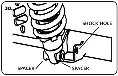
**20.** Install a spacer on each side of the lower Shockwave/Coilover. Slide the shock with the spacers installed into the mount on the lower StrongArm. You may need to jack the rearend up to line up the holes in the bushing with the 1/2" hole in the shock mounts and hold it in place while you install the 1/2" x 3 1/4" bolt and 1/2" Nylok nut. Tighten the upper and lower shock bolts.
