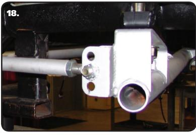
**18.** Install the other end of the Panhard bar into the bracket on the Passenger StrongArm using a 70013334 Spacer in each side of the R-Joint end. The **center** hole is the standard hole. The goal is to keep the panhard bar level as possible at **ride** height. If you decide to run the system higher or lower than the designed ride height the other 2 holes can be used to help keep the panhard bar level at **ride** height.
