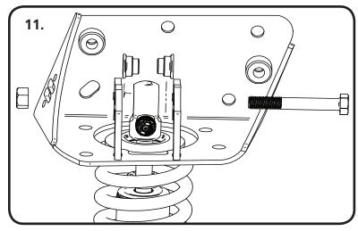
**11.** Install a spacer on each side of the upper Coilover. Slide the assembly into the upper mount from the bottom side. If your shock has an adjuster knob position it to the wheel side of the mount. Line up the hole in the spacers with the hole in the strap and insert 1/2" x 3 1/4" bolt and install 1/2" Nylok nut.
