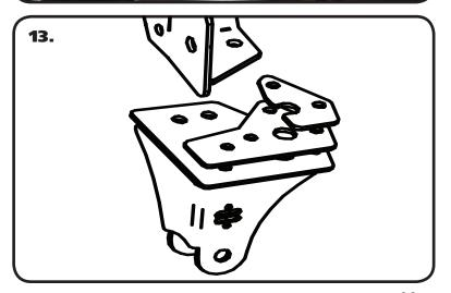
**13.** Bolt the new panhard mount to the bottom side of the frame on the drivers side. The panhard mount uses (2) spacers to mount it properly (See diagram #13 for reference). The new panhard mount is bolted in place using (6) 7/16" x 1 3/4" bolts, Nylok nuts and flat washers.
