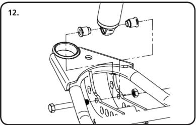
**12.** Install a spacer on each side of the lower Coilover. Slide the shock with the spacers installed into the lower control arm. Raise the arm up to line up the holes in the bushing with the 1/2" hole in the control arm straps and hold it in place while you install the 1/2" x 3 1/4" bolt and 1/2" Nylok nut. Tighten the upper and lower shock bolts to 75 fltbs.
