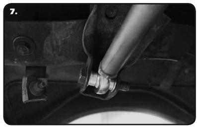
7. Install the panhard bar in the frame mount. It is installed with a Spacer on each side of the Heim. The Spacer is positioned with the small diameter against the heim. The large diameter of the Spacers should be against the mounting tabs. Install a 5/8" Flat Washer on a 5/8"-18 x 3 1/2" Hex Bolt and insert it through the Mount, Spacers and Panhard bar. With the Bolt installed, install a 5/8" Flat Washer on the threads followed by a 5/8"-18 Nylok Nut.
