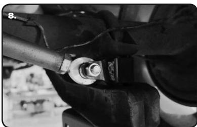
**8.** Repeat the procedure in step 7 on the axle side of the Panhard Bar. You may need to push the rear differential to one side or the other to get the Panhard bar lined up in the Mount.
