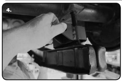
**4.** The kit contains 2 spacer blocks with one having the panhard mount welded to it. The spacers are installed between the axle and the trailing arm. The spacer block with the mount welded to it is installed on the passenger side with the mount positioned to the rear inside. Remove the OEM u-bolt and install the u-bolt supplied in the kit. Slide the spacer block onto the u-bolt followed by the OEM trailing arm.
