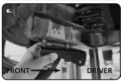
**6.** If you purchase the StreetGrip Shock Kit, install the lower mount at this time. The Mounts are installed on the U-Bolts, on the bottom side of the trailing arm. The shock mounting hole should be positioned with the hole to the front and to the inside of the truck. Once the Mount is installed, install a 3/4" Flat Washer and 3/4"-16 Nylok Nut on each leg of the U-Bolts. Tighten the Nylok Nuts to 350ftlbs.
