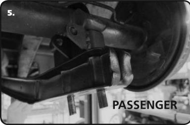
**5.** Diagram "5" shows the passenger spacer block installed. Note the position of the panhard mounting tabs.
