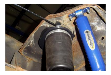
6. Hold the air spring assembly up to the coil spring pocket with the stud protruding through the hole in the center of the coil spring pocket. Place the 4" diameter washer over the stud and tighten with a 7/16" Nyloc nut and flat washer.
