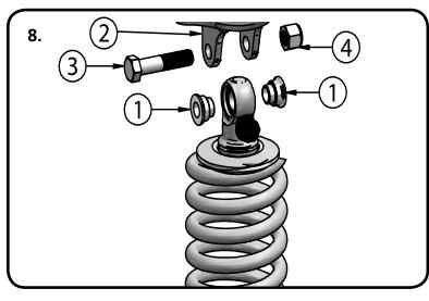
**8.** With the CoilOver assembled insert the upper spacers(1) into the upper shock bearings. With the spacers installed insert the CoilOver assembly into the upper shock mount(2). Align the holes in the bracket with the hole in the Shock spacers and insert the 1/2" Bolt(3) and secure with the 1/2" Nylok Nut(4).
