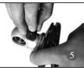
Slide the Derlin washer over the spring, Next slide the upper spring mount (90002222) over eyelet as seen in figure 4.
