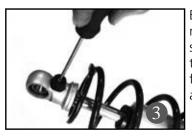
mount can be installed screw the adjuster knob on the upper eye mount to the firmest setting (clockwise) as seen in figure 3.
