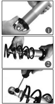
First using the supplied lower adjuster nut(90002222) thread the nut onto the shock from the top side as seen in figure 1
