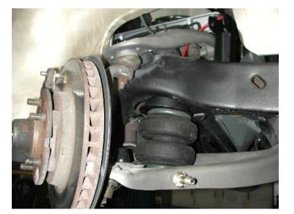
5. Place the assembly into the coil spring pocket with the stud sticking through the factory shock hole. Install 7/16" flat washer and Nylok nut onto stud.
