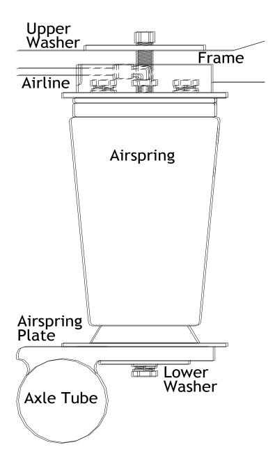
10. Check air spring clearance with exhaust and anything else that could rub against it. Abrasion will cause air spring failure and is not a warrantable situation.
