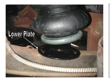
5. Place the lower air spring plate on top of the lower arm. Raise the axle up to the air spring and fasten with a 3/8" x 1" bolt, lock washer and flat washer.
