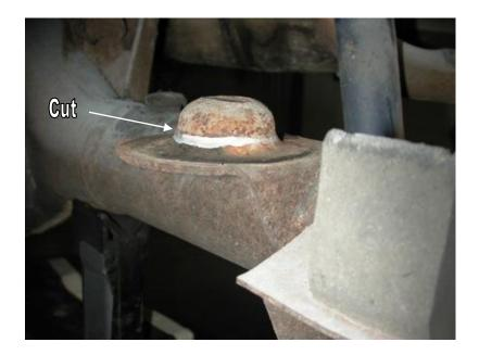
3. To allow the air spring to sit flat on top of the axle mount, the coil spring retainer must be cut down to about ¼" tall. Leave just enough of this retainer to locate the air spring roll plate, but make sure it is short enough not to contact the air spring piston.
