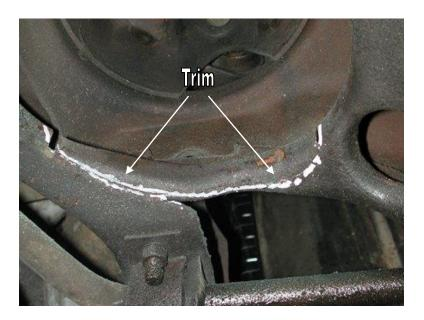
3. The front and outside lip of the coil spring pocket must be trimmed to allow clearance for the Shockwave. This is best done with a die grinder and a cut off wheel.
