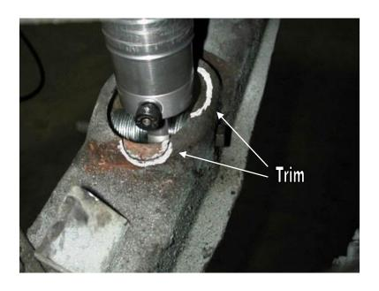
5. The lower control arm must be clearance as well to allow clearance for the shock body and the adjustment knob.
