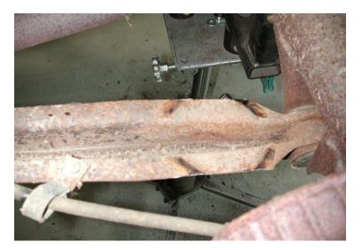
3. The lower coil spring retainer must be removed by cutting the welds. Grind all sharp edges smooth.
