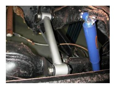
1. Attach shock T-Bar to frame using 5/16" x 1" bolts, Nylok nuts and flat washers.
