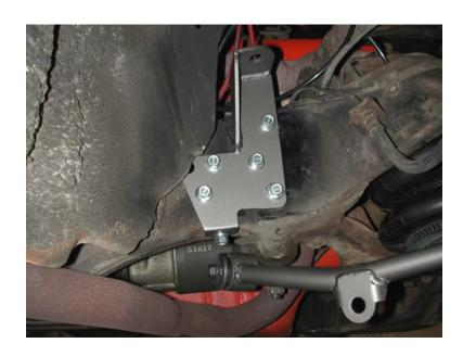
1. Position the upper shock mount on the frame so the hole in the bracket aligns with the hole in the side of the frame and the tab is against the bottom of the frame. You may have to trim some of the inner fender well for clearance. On manual shift cars you may have trim the bottom of the Z-bar clutch bracket on the driver's side.
