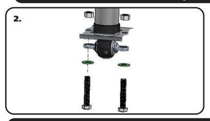
**2.** Attach the Trunnion to the OEM Control arm using the OEM hardware. It may be necessary to rotate the Trunnion to get it in the correct position. This can be done by sticking a screwdriver in one of the slots and spinning the trunnion in the shock bushing.
