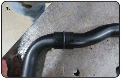
1. The Delrin Liner is split on one side to ease installation. We found it easier to install by opening up the Liner enough to slide it onto the end of the Sway Bar, then sliding it into position. It will open up and slide over the curves in the Bar. Install a Liner on each side of the Sway Bar in the approximate location they will need to be when installing the Sway Bar on the Car.
