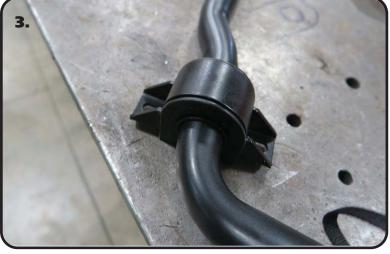
**3.** Install Bushing Straps Over the Poly Sway Bar Bushings.
