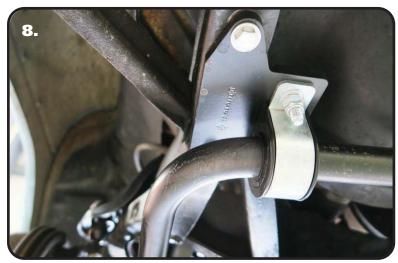
**8.** With the Delrin Liners/Bushings and Straps installed on the Sway Bar, put the swaybar in position on the 3/8" Bolts. Attach it using 3/8" Flat Washers and 3/8" Nylok Nuts. Do **NOT** Complete tighten the Hardware. It will be left partially loose until the End Links are installed.
