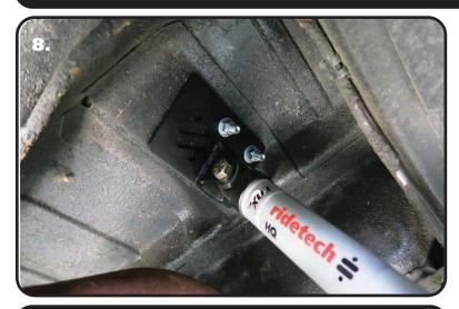
**8.** The Shock is mounted in the Upper Mount with the BODY UP. It is held in place with a 1/2"-13 x 2 1/2" Hex Bolt & 1/2"-13 Nylok with a 1/2" Flat Washer on each side of the bracket. **SKIP TO STEP #12**
