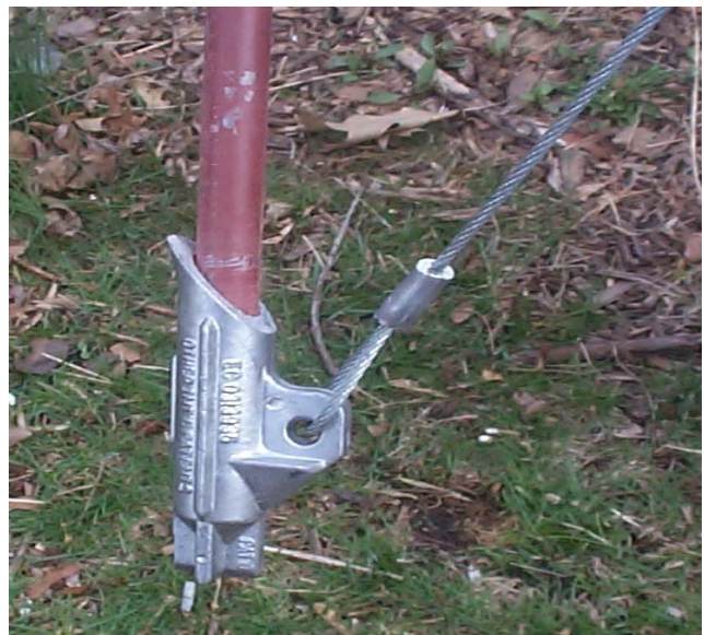
Drive Rod inserts into Anchor Head
