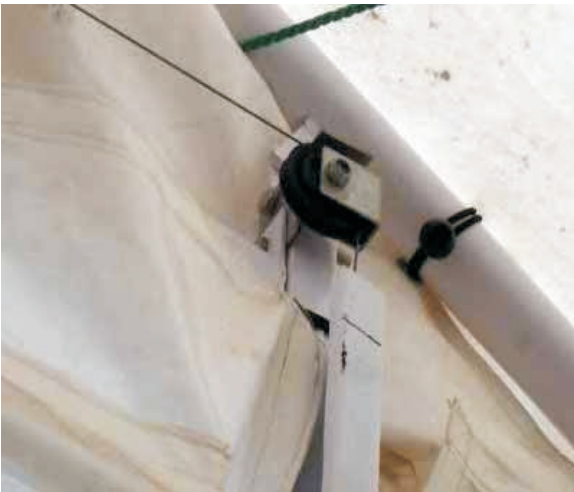
Single Door Pulley Farthest From Winch Assembly
