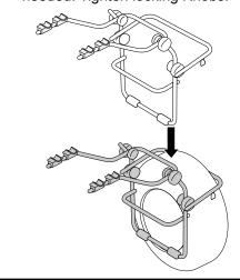
Secure the Bike Carrier in place. Use the Retaining Strap to secure the Carrier around the tire as shown.
