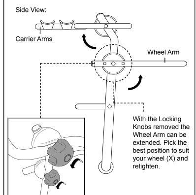
Place the Carrier onto the Spare Wheel of the Vehicle. Make any adjustments needed. Tighten locking Knobs.
