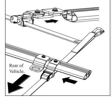
Wrap the snap hook end of the strap over the ladder runs. Snap the hook onto the hook bracket ensuring the safety latch is fully closed onto the hook. Pull the strap to tighten around the ladder runs. Check that the ladder is secure. To release the ladder, press the camlock latch and pull the strap back through the camlock, unhook the snap hook, if travelling with out a ladder, locate the snap hook onto the hook bracket.
