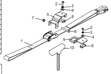
Remove the sportz leg if required. Slide the snap hook bracket and strap bracket into the end of the crossbar as per the diagrams. Position the camlock and hook bracket to suit the ladder, tighten the bolts with the allen key provided.
