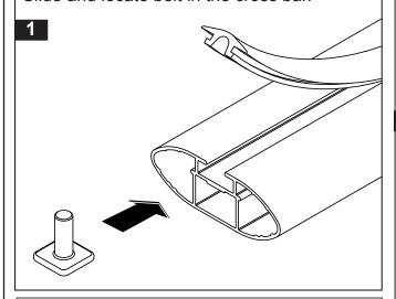
Locate bolt on cross bar. Place a flat washer and turn eye nut onto the end of each bolt. Tighten with the shank of a screwdriver. For secure tie off points ensure the eye nut hole faces the front and rear of the vehicle.
