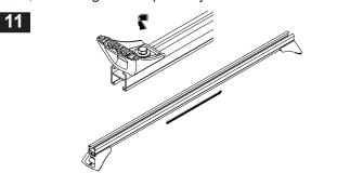
Check that the channel nut is fully located across the bar.
