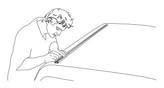
Mark end of tracks and mark the centre of the C-channel on both ends of each track. Move the track out slightly and use it as a straight edge to join the two points.
