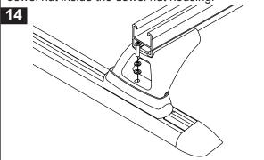
Using the security allen key provided tighten support leg attachment screws to secure the cross bars. Recommended tightening torque 3-4 Nm. **DO NOT OVER TIGHTEN.**
