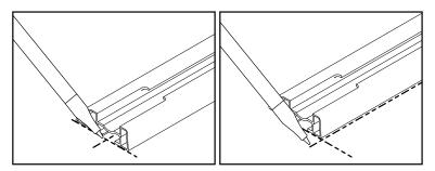
Mark and drill holes, as shown. Mark end holes 15mm in from end of tracks (the center of the T-bolt is placed 15mm from the end of the tracks). Spacing for T-bolt holes to be no greater than 280mm. Refer diagram. Vacuum fibreglass particles off canopy surface.
