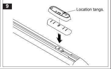
Insert the heavy duty leg assembly into the underside channel of the cross bar.
