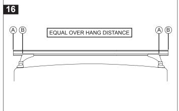
Tighten the cross bar attachment bolts. Recommended tightening torque 17-19 Nm. **DO NOT OVER TIGHTEN.** Check that the channel nut is located across the cross bar.
