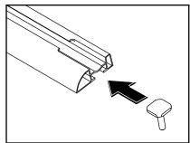
Install track end caps. Remove paper gasket from foam tape on underside of track. Place tracks onto canopy / hard tonneau. Ensure the cut outs are placed toward the rear of the vehicle. Double check that all T-bolts have o-rings fitted.
