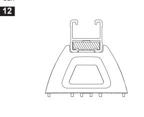
Insert the support legs into the mounting pads.
