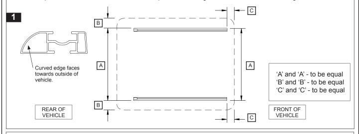
Position the tracks as close as possible to the outside edge of the canopy, this will ensure maximum strength. **Before** marking track holes, check on underside of canopy to ensure knobs have sufficient clearance to be located.
