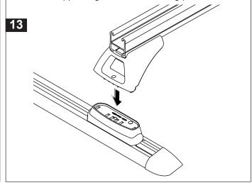
Place the M6 spring washer and M6 flat washer onto the M6 x 35mm security screw. Insert the M6 screw assembly through the support leg and screw into the dowel nut inside the dowel nut housing.
