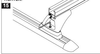
Check the cross bar over hang (A) (B) is equal on both sides, re-adjust if required.
