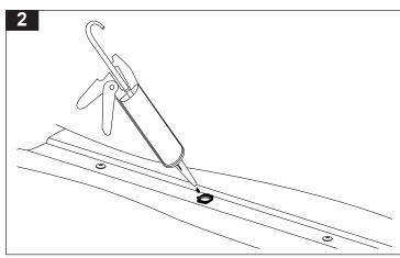
Apply silastic sealent in and around the holes you have removed the plugs from to eliminate water leaks.
