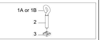
Screw the ladder peg into the channel nut, the channel nut grooves facing the rounded end of the ladder peg.
