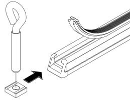
Position the ladder peg, tighten the ladder peg to secure. Check that the channel nut grooves are located in the crossbar section. Trim rubber buffer strip to suit.
