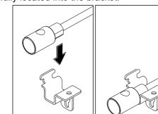
Insert the T-shaped lugs on the brackets into the underside of the crossbar. Turn the cable lock and bracket assembly so that the lugs engage the crossbar and the channel nut goes up into the crossbar recess.
