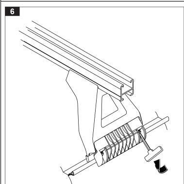
Progressively tighten lower clamp screws to secure the roof rack to the gutter. Repeat the tightening process on each side of the vehicle. Tighten M6 screws to 3-4 Nm. Do not over tighten.
