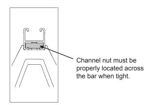
Measure for equal crossbar overhang. Hold the leg against outer edge of the gutter. Use a 5/8" or 16mm spanner and tighten M10 bolt & channel nut to 13-15 Nm. Do not over tighten.
