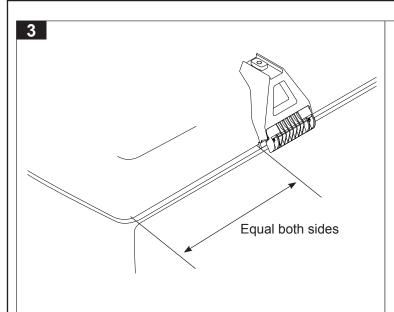
Position the legs parallel across the vehicle. Measure from same point each side of the vehicle. Rotate the clamp underneath roof gutter lip. The clamp must be fully located into the corner of the gutter lip. Finger tighten clamp screws.
