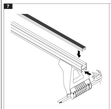
Insert end caps and buffer strips into crossbar. A rubber mallet may be used to knock the end caps in. Re-check all attachment bolts and screws after fitment.
