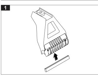
Loosen leg clamp screws. Install the rubber boot.
