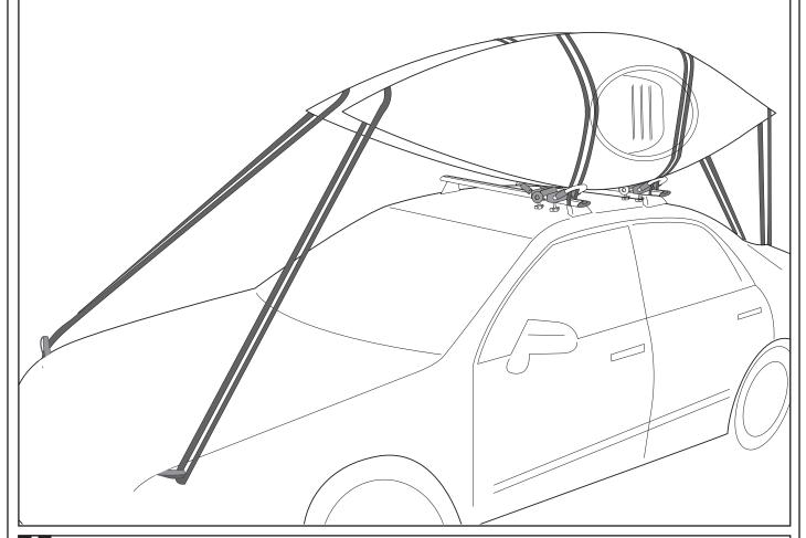
When not in use, fold straps over and hide them under the bonnet of the car. Avoid the straps flapping as they may cause paintwork damage.
