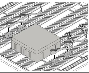
Pull the strap through the Cam Buckle as shown.
