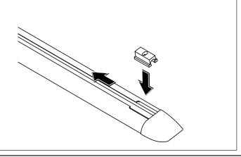
Position base pad and top pad over dowel nut housing. Note: The four location tangs on the top pad face toward outside of vehicle.
