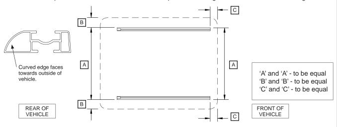
Position the tracks as close as possible to the outside edge of the canopy, this will ensure maximum strength. Before marking track holes, check on underside of canopy to ensure knobs have sufficient clearance to be located.
