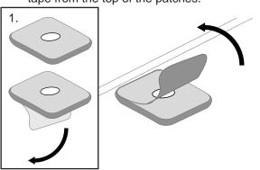
Install track end caps. Remove paper gasket from foam tape on underside of track. Place tracks onto canopy / hard tonneau. Ensure the cut outs are placed toward the rear of the vehicle. Double check that all T-bolts have o-rings fitted.
