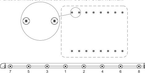
Place dowel nut housing in the large cut out in track. Slide along to desired position.
