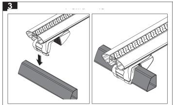
Gasket will flare out when pressure is applied creating a seal.
