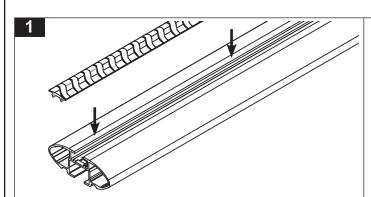
Press the rubber buffer strip into the top of the cross bar.
