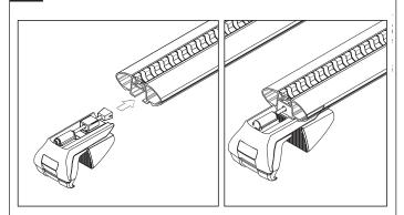
Slide each leg assembly into the end of the cross bar.
