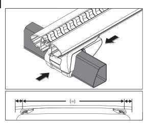
Pull the inner and outer clamp legs together around the rails. Adjust the cross bar so that the overhang is equal both sides. **Do not fully tighten as final tightening occurs later.**
