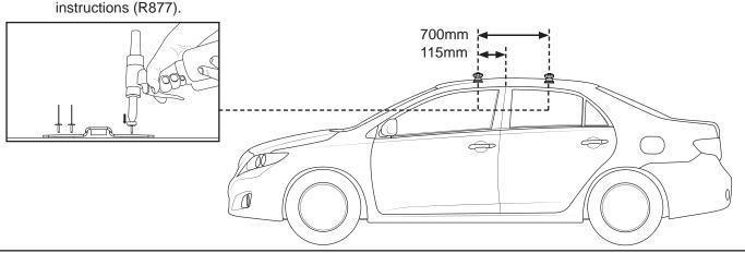
Note Vortex crossbars can be cut to length to fit this vehicle. Measure the desired length out from the centre of the Vortex Bar and create a reference with a marker. Carefully cut the bar at these markings using a Saw with an Alloy Cutting Blade.
