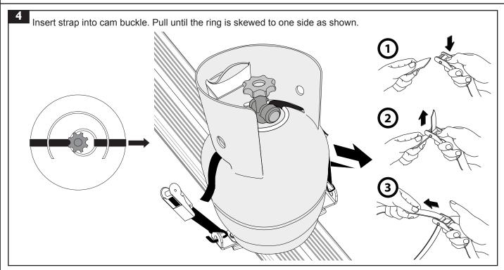
Insert strap into rachet as shown (1). Pull strap tightly (2). Tighten the ratchet lever till the gas bottle is secured to the alloy tray (3 & 4). Repeat steps 3 and 4 till tight. Ensure that the ring is concentrically aligned as shown.
