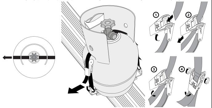
To undo the straps, first undo the ratchet lever as shown. Then undo the cam buckle as shown in step 4 in reverse.
