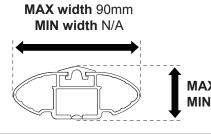
MAX height 33mm MIN height 22mm
