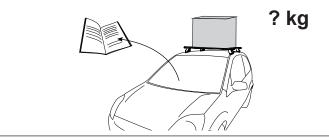
When these roof racks are to be used on a vehicle that is driven off sealed roads, the manufacturer maximum roof load rating (to be found in the vehicles User Manual) should be *divided by 2*. Do not forget to subtract the complete crossbar system weight from your maximum carrying capacity.
