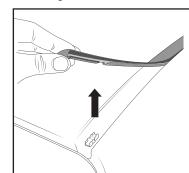
Be sure to check vehicle specific instructions for removing Ditch Mould. Some vehicles may use clips to hold the Mould in place. Care is needed as to not damage them in removal.
