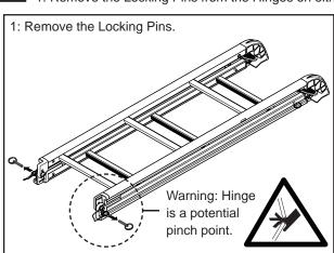
Open the Ladder. Be sure to replace the Locking Pins. Failure to do so could result in injury or damage to the vehicle.
