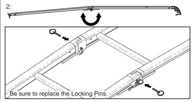
Slide the Top of the Ladder over the installed Hook Brackets. Be sure the Ladder is seated correctly in the Brackets. If the Ladder position is satisfactory, tighten the Brackets into place with the Allen Key provided.
