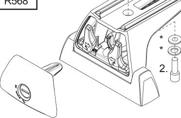
Quick Mount Spacers can be combined to achieve a desired height. 5mm
