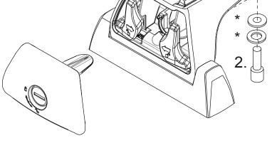
\*Fix the Quick Mount Spacer to the Leg using the hardware in the leg kit. The bolts found in the spacer kit will replace the original in the leg kit.
