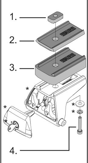
Note: Max Spacer height 30mm
