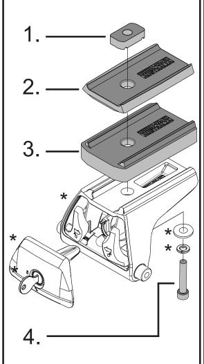
Note: Max Spacer height 30mm
