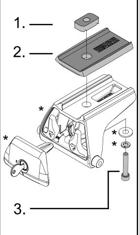
Note: Max Spacer height 30mm
