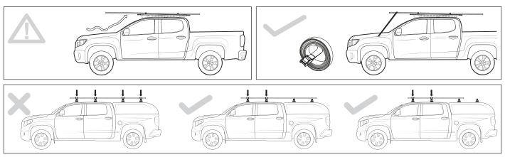
Max system load capacity (incl. system weight), refer to vehicle specific fit sheet.
