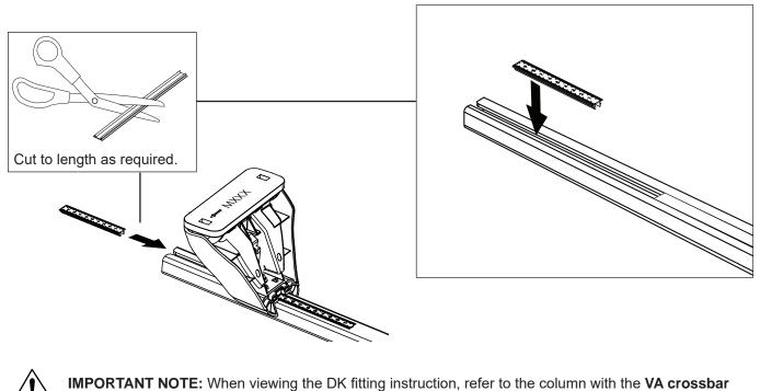
**IMPORTANT NOTE:** When viewing the DK fitting instruction, refer to the column with the **VA crossbar** and not the column of Alloy Eurobar as shown below.
