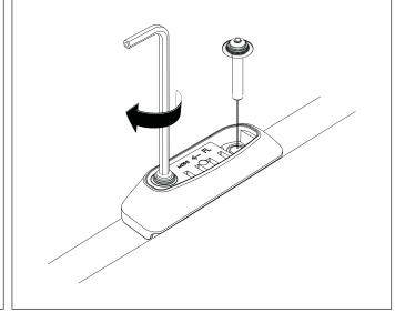
When crossbars are not in use, install the pad mount cover plates as shown.
