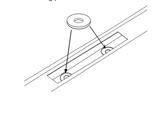
Insert the mounting pad through the cover trim and into the roof gutter at the positions shown on the roof layout (step 3). Ensure that the arrows on the pads are pointing to the front of the vehicle and the holes in the washer gasket are aligned with the mounting pad holes.
