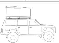
When these roof racks are to be used on a vehicle that is driven off sealed roads, the manufacturer maximum roof load rating (to be found in the vehicles User Manual) should be *divided by 1.5.* Do not forget to subtract the complete crossbar system weight from your maximum carrying capacity.
