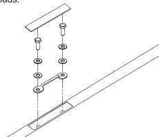
Each mounting pad is identified with a part number, position code and direction arrow. The arrow must point toward the front of the vehicle.
