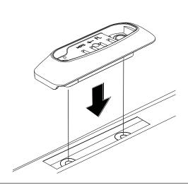
Insert the assembled M8 screws through the mounting pads and screw into the nutserts in the vehicles roof. Tighten all screws using the allen key provided. Recommended tightening torque 15Nm. **DO NOT OVER TIGHTEN.**
