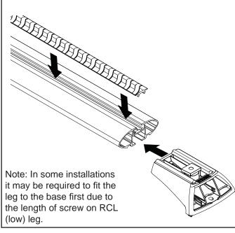
Fix the Crossbars to the vehicle specific Base Kit that has been purchased, using the Allen Key provided.
