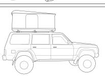
When these roof racks are to be used on a vehicle that is driven off sealed roads the maximum load rating must be divided by 1.5.
