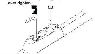
When crossbars are not in use, remove and install the pad mount cover plates using the M6 hardware provided.
