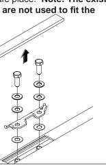
Place the 10mm large o-rings onto the protruding plastic tubes.
