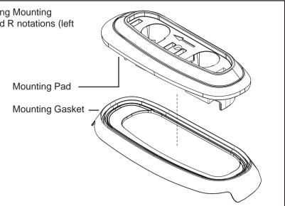
Place each pad into its position as stated in the previous step. Check to make sure the rubber skirt does NOT fold or twist when placed on the roof. It must flare out over surface of the roof.
