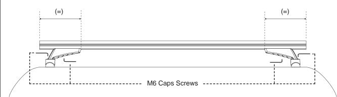
Insert the Underbar Strips into the slots either side of the installed Leg. Cut to length as required.
