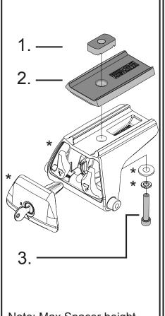
Note: Max Spacer height 30mm
