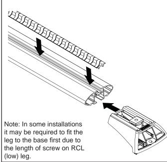
Fix the Crossbars to the vehicle specific Base Kit that has been purchased, using the Allen Key provided.
