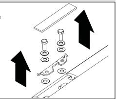
Place the foam covered mounting pad washers (item 20) over the plastic tubes in the roof channel. Make sure they are fitted neatly around the plastic tubes.
