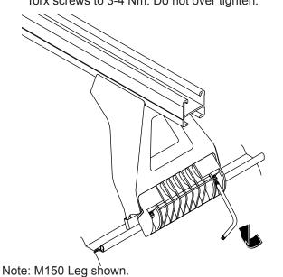
Insert end caps and buffer strips into crossbar. A rubber mallet may be used to knock the end caps in.
