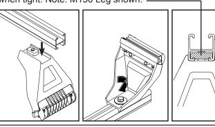
Measure for equal crossbar overhang. Hold the leg against outer edge of the gutter. Use a 5/8" or 16mm spanner and tighten M10 bolt & channel nut to 13-15 Nm. Do not over tighten.
