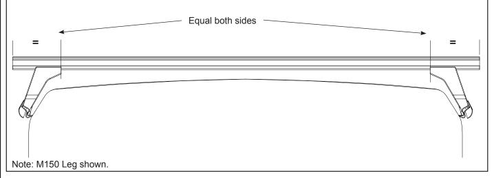
Progressively tighten lower clamp screws to secure the roof rack to the gutter. Repeat the tightening process on each side of the vehicle. Tighten M6 Torx screws to 3-4 Nm. Do not over tighten.
