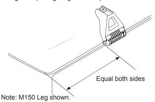
4 Place crossbars onto legs. Push the leg attachment bolt up and turn so the channel nut is fully located across the inside of the bar. Finger tighten M10 bolt at this stage.
