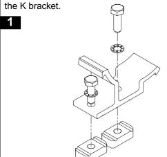
Turn the bolts so that the channel nuts are fully located across the crossbar. Position the K bracket to suit the conduit pipe being used. Tighten the bolts. Check that the channel nuts are fully located across the crossbar after tightening.
