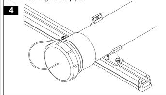
Slide the upper C bracket onto the K bracket.
