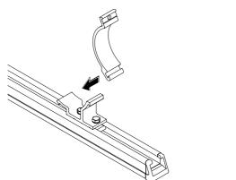
Place the conduit pipe onto the K bracket with lower C bracket resting on the pipe.
