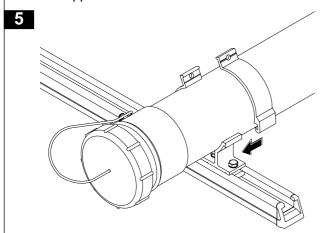
Holding the upper C bracket against the pipe insert the hex bolt flat washer and nyloc nut. Do not fully tighten the nut. Adjust the conduit pipe to suit the multi slide layout. Tighten the clamp bolt. Check that the conduit pipe is secured.
