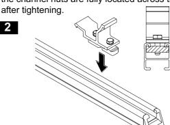
Slide the lower C bracket onto the K bracket.
