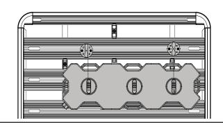
Place the Rotopax onto the pack mounts. Tighten all four
