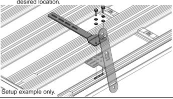
Fix the rear of the Bracket in place by sliding the M6 Channel Nut into the 'C' Channel of the Platform and aligning with the corresponding hole on the Bracket. Slide the M6x20 Hex Bolt, with the M6 Spring and Flat Washers from this kit, into the channel nut. Tighten with a 10mm socket.
