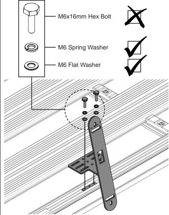
Using the item 2 and M6 Spring and Flat Washers from the previous step install the Recovery Track Support Bracket as shown. Tighten with a 10mm socket in the desired location.
