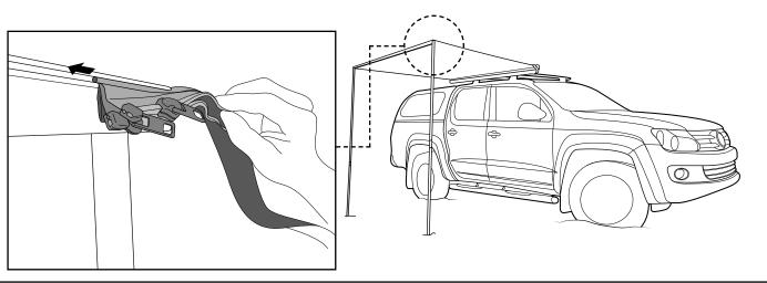
Attach the Fly Extension first to the Sunseeker using the Dual Zipper Insert. The fold over the Sunseeker while attaching the Tag-A-Long second.
