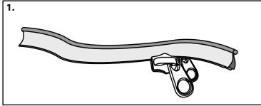
Install the Double Zipper insert into the Sunseeker Awning as shown.
