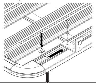
The Brackets can slide into the Pioneer in a lowered position. Note, the awning will sit in as lightly lower position on the vehicle. Tighten with a 13mm wrench.
