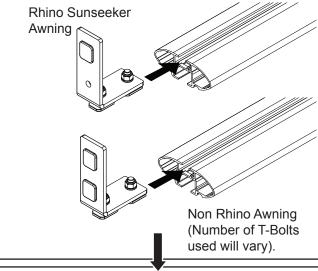
The Brackets can slide into the Aero Bar in a lowered position. Note, the awning will sit in a slightly lower position on the vehicle. Tighten with a 13mm wrench.
