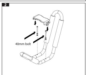
The 40mm bolts will not protrude out of the bottom. The carrier is now ready for the C-channel fitment
