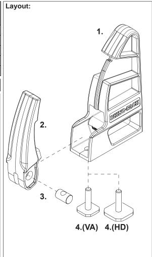
Insert the assembly created previously into the main body.
