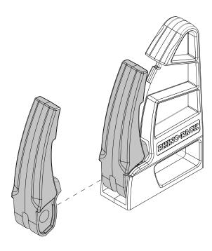
Insert the T-Bolt into the main assembly. Finger tighten half way.
