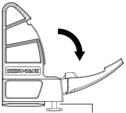
**Note:** Opening the lever leg lengthens the T-Bolt thread.
